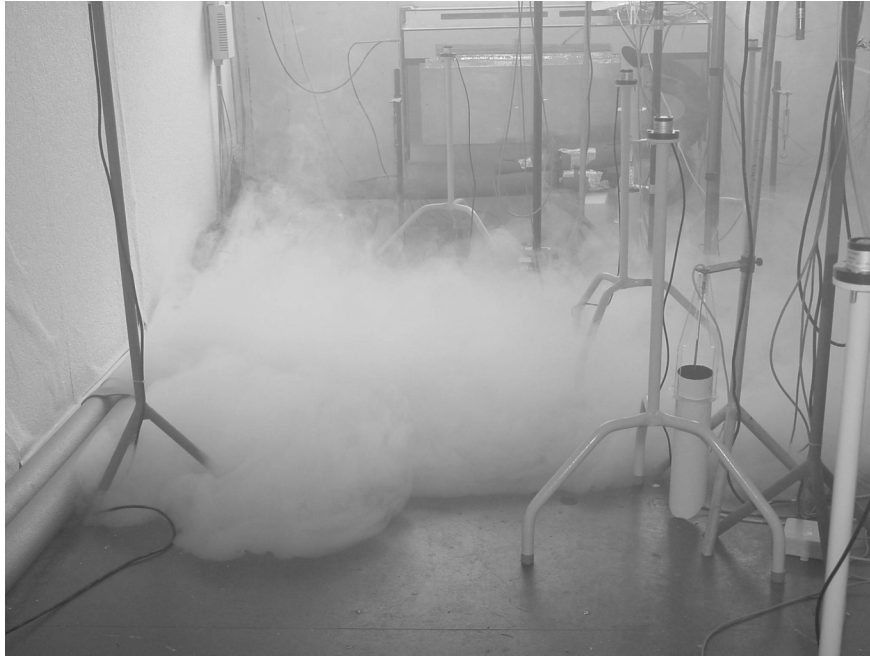
Figure 5: Visualization of air flows by means of artificial fog
